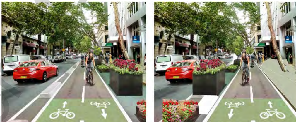
Figure 10: Possible use of planter boxes (right) to separate bikeways from motor vehicle traffic.
