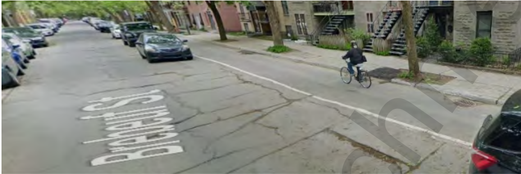
Figure 5: Parallel parking on both sides of a street, with a bikeway protected by the parked cars.
